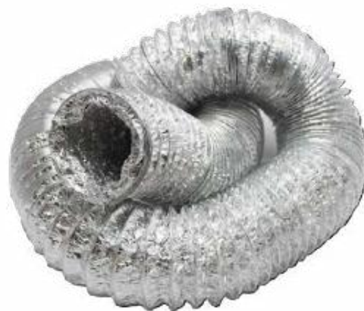
CFD PVC combine flexible duct constructure: PVC+PET +alu foil temperature rating -30 to 150°C fire resistant standard length: 10m
