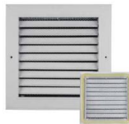
SG-FB: without metal screen SG-FBN: c/w metal screen material: aluminum standard color: white Ral9016 / 9010 standard size: 150x150 200x200, 250x250, 300x300, 350x350 (mm) customized size upon request
