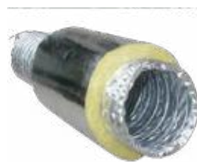
IFD-S&D single/double layer alu foil duct + fiberglass+alu foil jacket temperature rating -30 to 150°C fire resistant standard length: 10m
