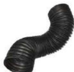
FC-CFD Material : PVC Constructure: double layers PVC + metal wire Temperature rating:-30 to 150°C Standard length: 10meters
