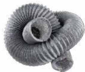
CFD PVC combine flexible duct constructure: PVC+PET +alu foil temperature rating -30 to 150°C fire resistant standard length: 10m
