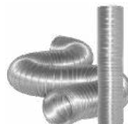
IFD-USR6/R8 Pink fiberglass insulated flexible duct PET inner duct + R6/ R8 pink fiberglass Insulation+aluminum foil jacket, Temperature rating:-30 to 150°C fire resistant Standard length: 10m
